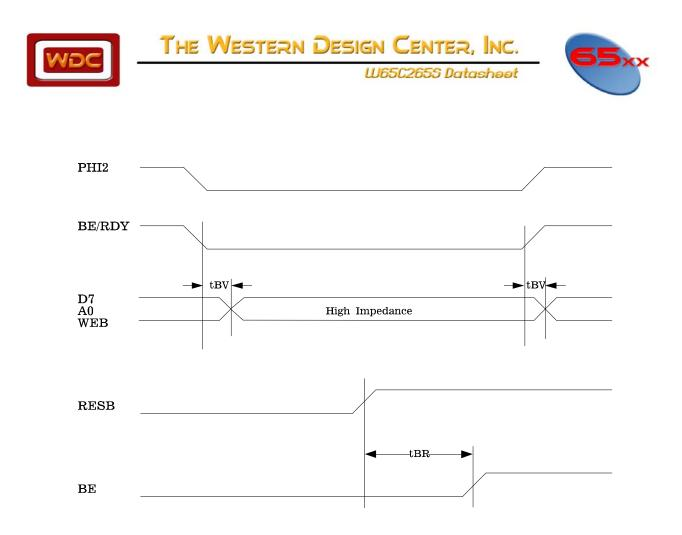
Figure 3-3 AC Timing Diagram #3
