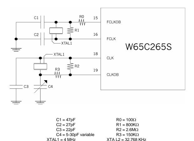
Figure 4-8 Oscillator Circuit
