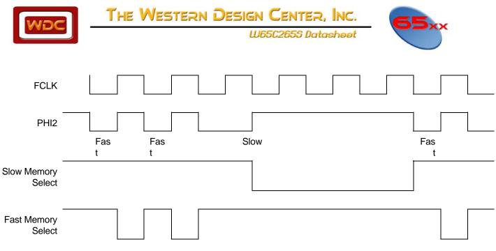
Figure 1-15 System Speed Change Timing Diagram
