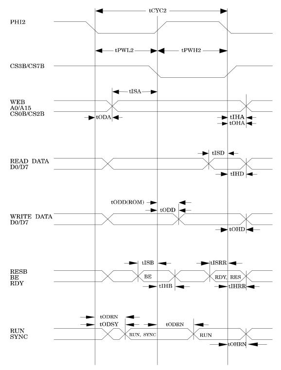
Figure 3-1 AC Timing Diagram #1
