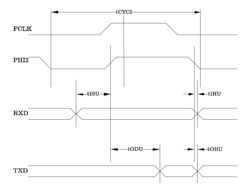
Figure 3-4 AC Timing Diagram #4
