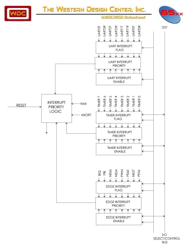
Figure 4-2 W65C265S Interrupt Controller Block Diagram
