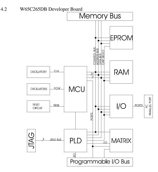
Figure 5-7 W65C265DB Developer Board
