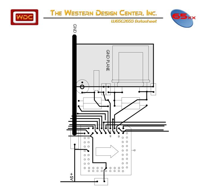
Figure 4-9 Circuit Board Layout for Oscillator Circuit
