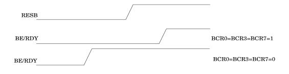
Figure 1-1 BE Timing Relative to RESB Input
