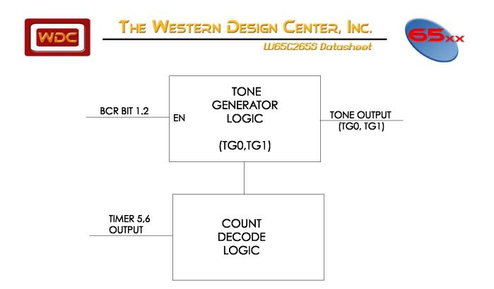
Figure 4-6 W65C265S Tone Generator (TGx) Block Diagram
