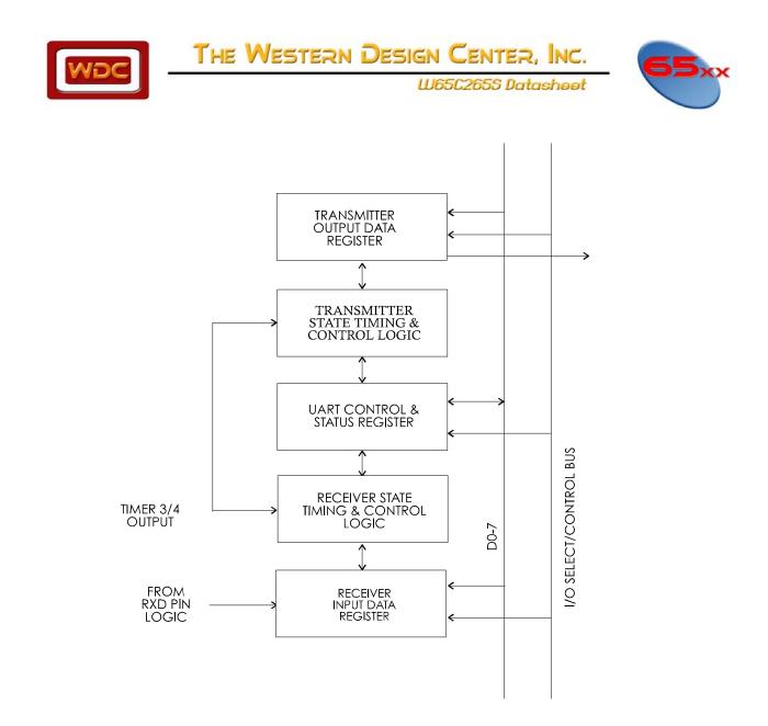
Figure 4-4 W65C265S UART Block Diagram
