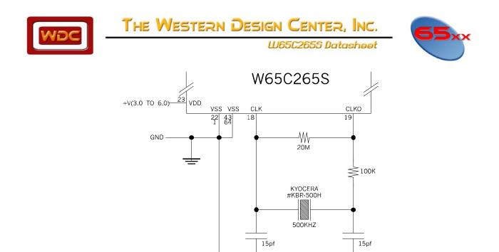
Figure 4-10 W65C265S Resonator Circuit
